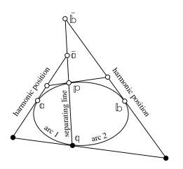
Figure 4: Biarc construction.
